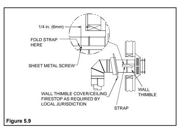
**Note:** The attachment from the vent pipe to the vent termination cap must be sealed with silicone. Termination caps shall not be recessed into a wall or siding.
